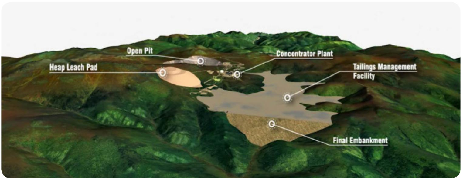
The mine has a total of 965 million tonnes of proven and probable Mill ore reserves and 157 million tonnes of proven and probable Heap Leach reserves. The open pit will ultimately occupy an area of approximately 300 hectares and will extend to a depth of approximately 600 metres.
